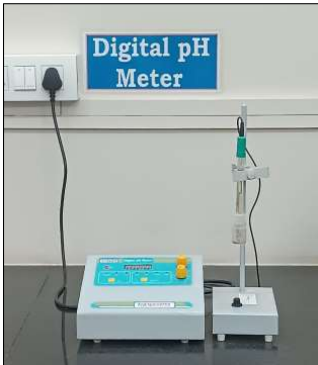
Name of instrument: Analab Scientific Digital pH/mV meter
