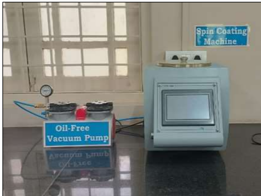
Name of instrument: Milman Table Top Spin Coater
