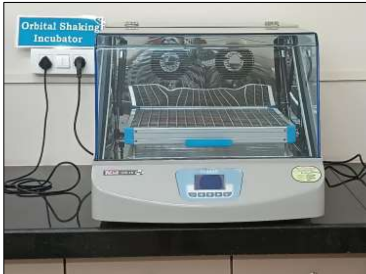
Name of instrument: REMI CIS- 18 PLUS orbital shaking incubator
